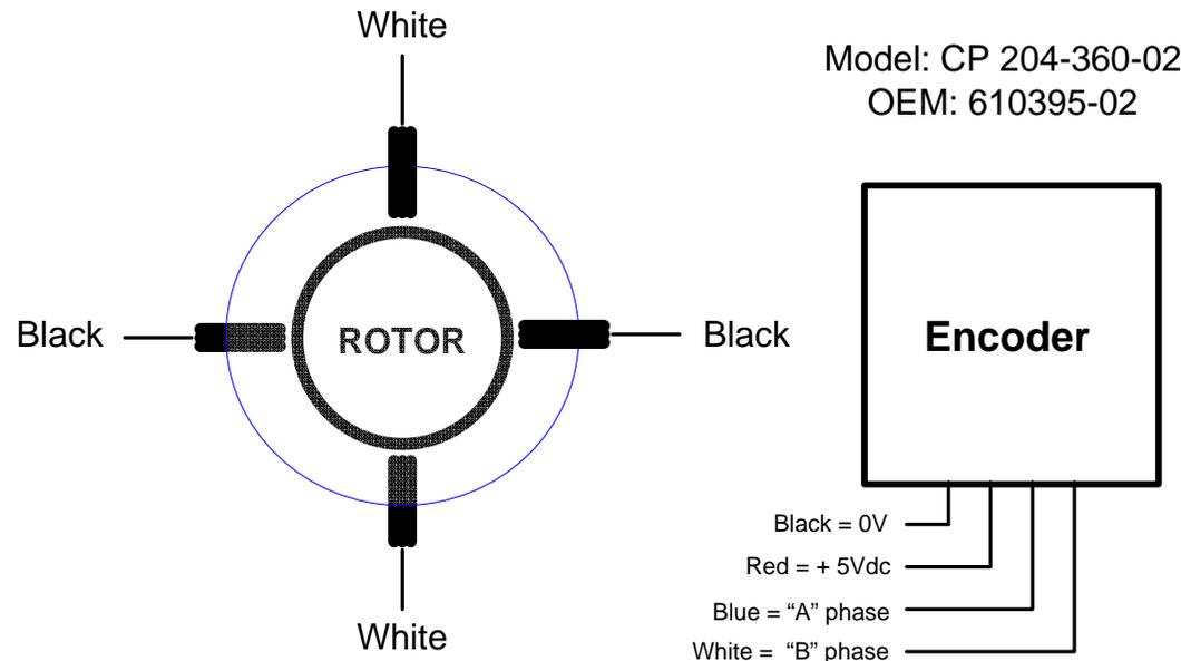
**Note:** from a Gecko-320 this motor delivers 1000rpm when 'speed' set to xxxxpps
