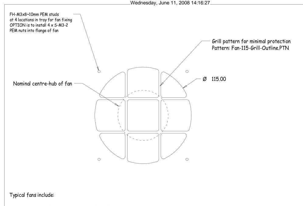
Sanyo - 1095089 (230Vac-50Hz-0.06A) 5 blade ball-bearing - 1" thick - alloy-body -impedance protected.
