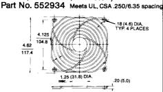
Material: Center Disc: .03 (0.76) THK. C.R.S. Wire Rings: .062 (1.57) DIA. STEEL Supports: .080 (2.03) DIA. STEEL Finish: Bright Zinc Plate with Chromate Treatment
