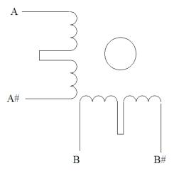
2 center wires of each coil connected (insulate connection)
