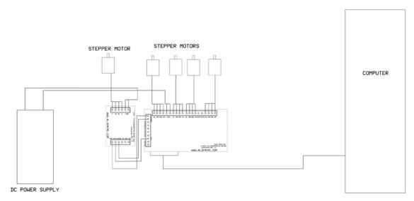
Note: Power Connection is not daisy chained (power connection is made directly from original power source
