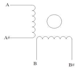
Each wire is connected to its corresponding terminal block location (i.e. A# wire is connected at **A#** location).
