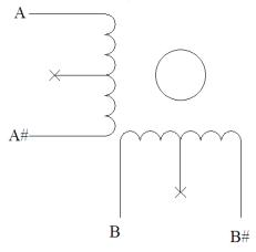
Center wire of each coil not connected (insulate termination)
