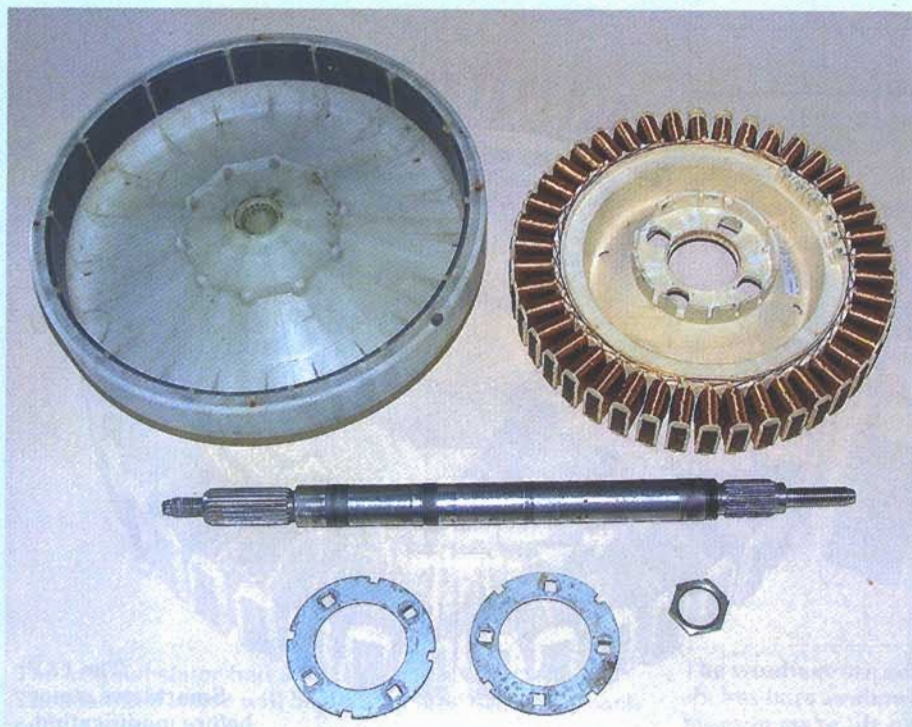
Inside the Fisher & Paykel Smartdrive washing machine motor – top left is the magnet hub, top right the stator, centre is the drive shaft, while at the bottom are the retaining plates and nut. We need all these parts for our windmill.
