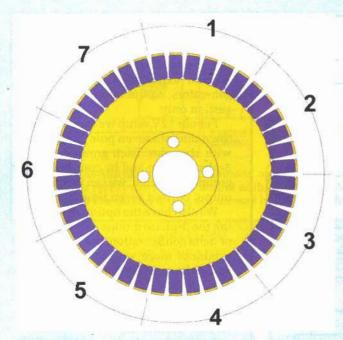
The original stator had 3 sections, each with 14 poles. The modified stator will be divided into 7 sections, each with 6 poles.
