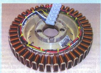
Fit a terminal strip to the finished stator. This makes it easier to change from star to delta configuration.
