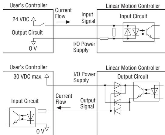
The linear motion controllers (EZSII, SPV, EZCII, EZA and PWAI Series) adopt an I/O specification that allows the controller to be used with either the NPN or PNP specification by changing the wiring.
