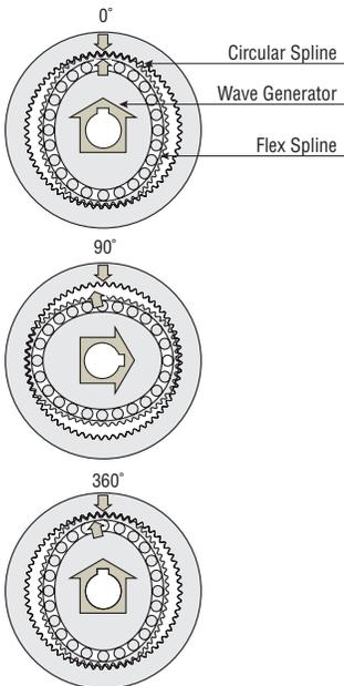
Combines three basic parts. The flex spline is bent into an oval shape by the wave generator. The teeth at the long axis of the oval mesh with the circular spline, while the teeth at the short axis of the oval are completely separate from it.
