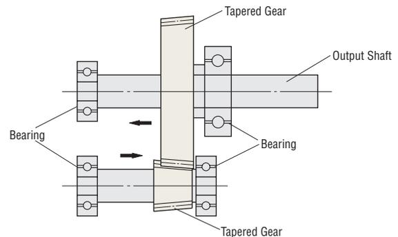
Structure of TH Gear's Final Stage
