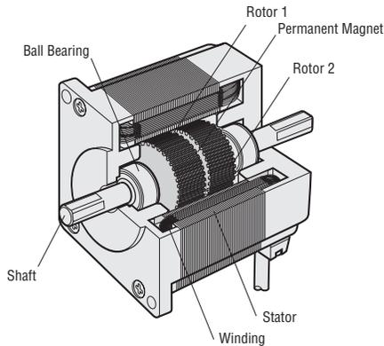
Motor Structural Diagram: Cross-Section Parallel to Shaft
