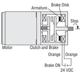
The figure below shows the relationship between the action of the motor shaft and output shaft and the state of excitation of the clutch and brake coils.
