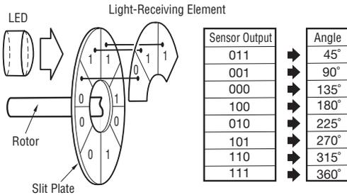
Capable of detecting absolute position within one rotation of the servo motor, the absolute encoder outputs the absolute position of the rotation angle.
