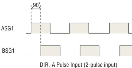
ASG1 output: Pulses corresponding to linear slide operation are output.
