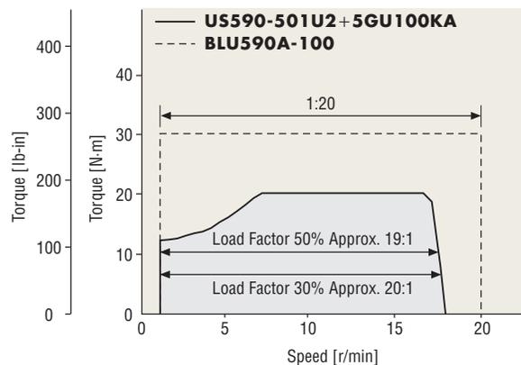
The maximum permissible torque of the **5GU100KA**, which has a gear ratio of 100:1, is 20 N·m (177 lb-in). The speed ratios at load factors of 30% and 50% are shown in the table below:
