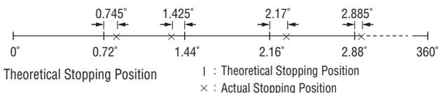
The stop position accuracy is within  $\pm 3$  arc minutes ( $\pm 0.05^\circ$ ), but only under no load conditions. In actual applications there is always the same amount of friction load.
