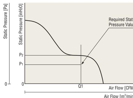
Fig. 6 Air Flow – Static Pressure Characteristics
