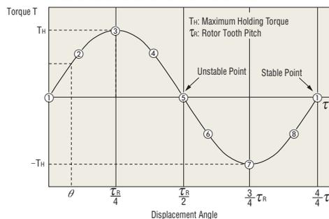
Angle – Torque Characteristics
