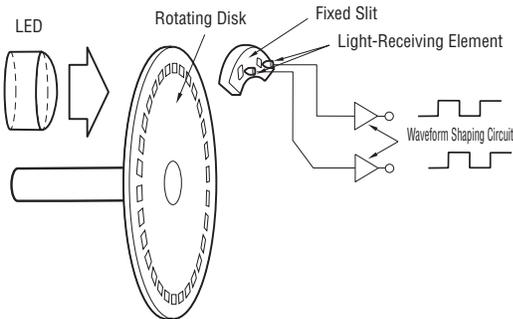
Capable of detecting the rotation, speed and rotation direction of the servo motor, the incremental encoder outputs the pulse with respect to the change portion of the rotation angle.
