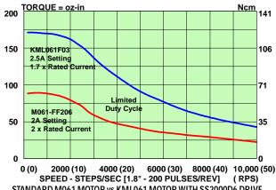
STANDARD M061 MOTOR vs KML061 MOTOR WITH SS2000D6 DRIVE
