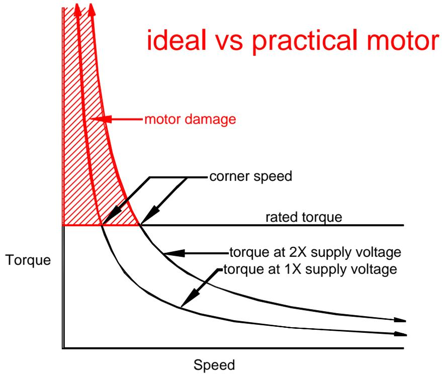
To prevent this, the drive must be set to limit the motor current to its rated value. Because torque is proportional to current, motor torque is constant from zero speed to the corner speed. Above the corner speed, motor current is limited by the motor's inductive reactance.
