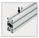
Where possible, profiles should be installed so that the largest section dimension opposes the load in order to achieve the maximum flexural strength.
