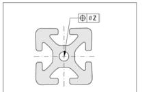
The hole position tolerance depends on the number of core bores and the profile contour.
