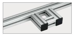
Avoid breaks in the supporting profile when installing additional attachments; the benefits include greater stability, fewer cuts, fewer connections and reduced assembly time.
