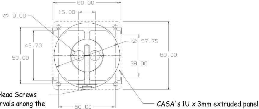
M4  $\times$  30mm Pan Head Screws at 50~75mm intervals anong the certral axis of assembly with 10mm OD  $\times$  0.9 Washer (or subchassis) + Spring Washer under the head
