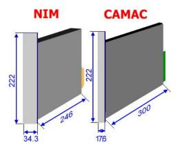
NIM is the perfect standard for small and flexible setups for high resolution measurements with analogue electronics (amplifier, high resolution analog to digital converter), timing modules, noise sensitive electronics as well as for low / high voltage supplies.
