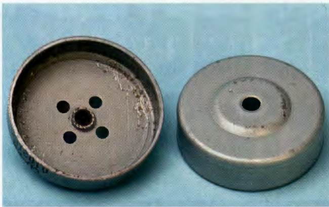
Standard sized bells ready for modification. Note the difference in heights. As long as you have enough material to safely glue the magnets to, any sized bell can be used. Also note the lip on the inside of the centre hole – this must be removed as described in the text.
