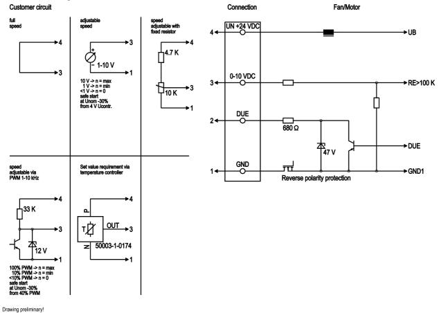
Conn. Designation Color No. Function/assignment 4 Un +24 VDC Power supply 24 VDC, maximum ripple 3.5% 1 red 0-10 VDC 3 Control input Re > 100 K 1 yellow Tach output, 2 pulses per revolution, Isink max = 10 mA 2 DUE white 1 GND 1 1 blue Reference ground
