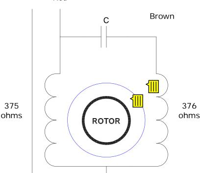
C is typically 1 to 4uF. Higher value gives higher torque but increased operating temperature. Care needed not to overheat motor.
