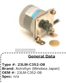
Frame: NEMA 23 Steps: 200/rev (1.8 Degrees per full-step or finer with micro-stepping) Current: 1.3 Amp Volts: 3.9 Vdc Torque: \_\_\_\_ Nm @ \_\_\_A (\_\_ oz.in.) Resistance: 3 Ohms / phase (nominal) Inductance: 4.3 mH / phase (nominal) Connector: 6 way x 0.1" (if fitted) Wires: 6 wire (up to 230 mm nominal) Shaft: 6.35mm dia x 19mm long Shaft-Detail: Plain Size: 57 x 57 x 52mm (nominal)
