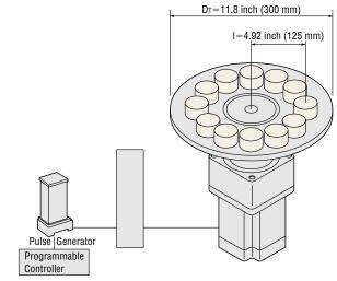
$D_{T} = 11.8 \text{ inch (300 mm)}$ Diameter of index table: Index table thickness:  $L_{T} = 0.39$  inch (10 mm)
