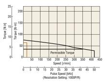
Select a motor for which the required torque falls within the pull-out torque of the speed-torque characteristics.
