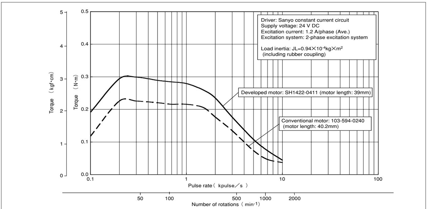
Fig. 5 Comparison of Torque Characteristics
