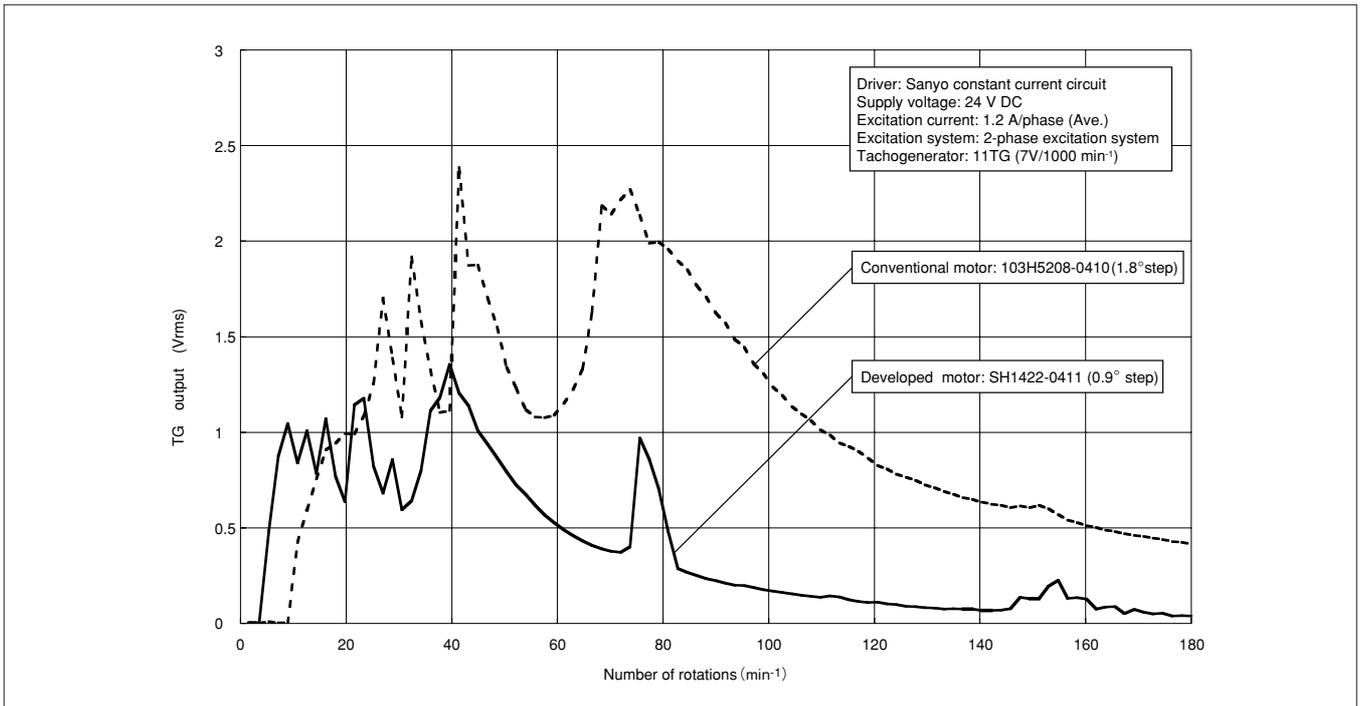
Fig. 4 Comparison of Speed Fluctuations in Basic Step Angle 0.9° and 1.8°
