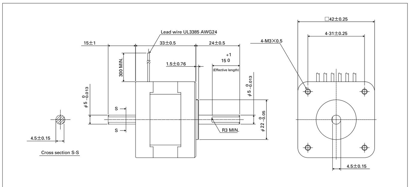
Fig. 2 External dimensions of the 2-phase 42mm Sq. 0.9° stepping motor "SANMOTION F"
