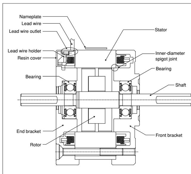
Fig. 3 Motor Structure
