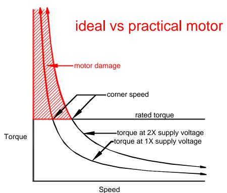
To prevent this, the drive must be set to limit the motor current to its rated value. Because torque is proportional to current, motor torque is constant from zero speed to the corner speed. Above
