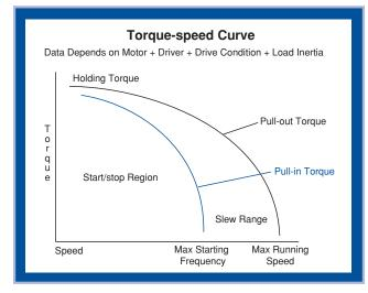
Torque/speed curves have torque on the Y-axis, measured in N-m (in this catalog), and speed on the X-axis, measured in PPS (pulses per seconds) or Hz.
