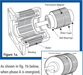
when phase A is energized, the windings at 12 o'clock and 6 o'clock are north poles, and the windings at 3 o'clock and 9 o'clock are south poles. The windings at 12 and 6 would attract the teeth of the magnetically south end of the rotor, and windings at 3 and 9 would attract the teeth of the mag-
