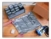
1. Remove the bag from the Instapak® Quick™ warmer, unfold it and lay it on a flat surface.
