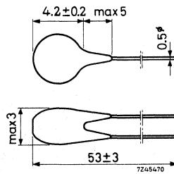
These varistors feature low capacitance and are for use in colour television and for protection of aerial inputs of car radios.
