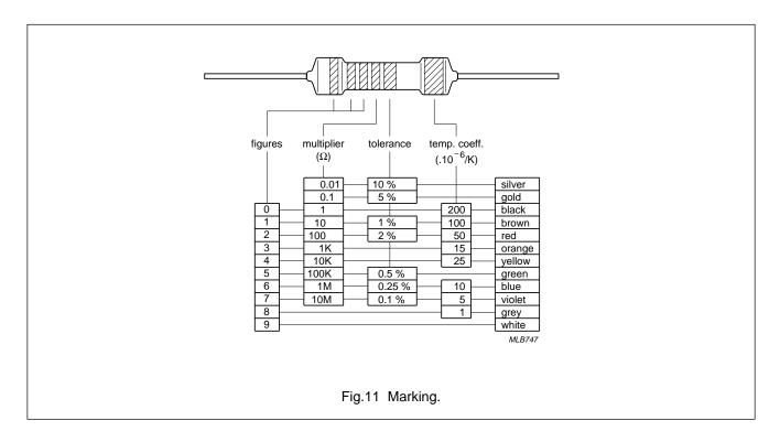
The **resistance code** consists of either three or four bands and is followed by a band representing the **tolerance**. The **temperature coefficient** is to the right of the tolerance band and is usually positioned on the cap (MRS types), as a wide band. When five or six bands in total are used, the last band will always be the wider one.
