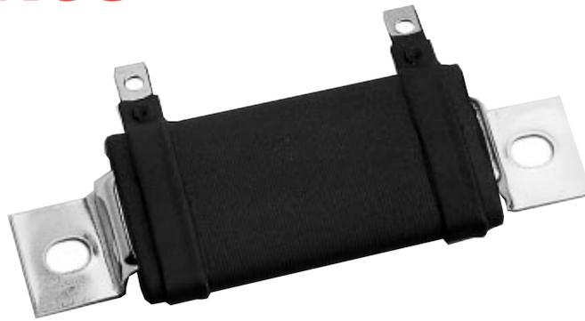
The FRW Series is designed for vertical or horizontal mounting, either singly or in stacks. Non-magnetic mounting brackets extending through the resistor allow easy and economical mounting. They also aid in heat distribution along its entire length and serve as conductors to transfer internal heat to the chassis.
