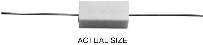
The PGR-T Series resistors extend the resistance range of the PW series with another inorganically filled ceramic boat type resistor. The PGR-T is entirely **flameproof** for use wherever MIL style power resistors are not mandatory and an industrial grade resistor is desired. The main flameproof characteristics are:
