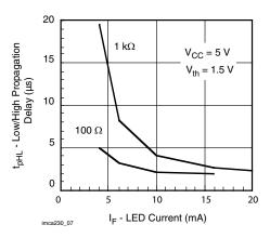
Fig. 7 - High to low Propagation Delay vs. Collector Load Resistance and LED Current
