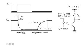
Fig. 8 - Switching Timing Waveform and Schematic
