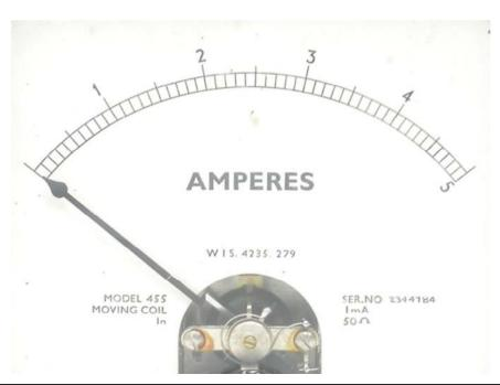
The formula for calculating the required current shunt resistance RS (Ohms) to enable a meter with a full-scale sensitivity of Im (Amps) and internal resistance Rm (Ohms) to measure Ifs (Amps) is:
