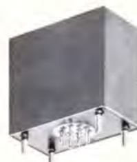
Bolometer transformer. Primary 10 ohms, secondary 530K ohms, 230:1 ratio, response from \frac{1}{2} Hz to 25 Hz. 120 db magnetic shielding, to 25 Hz. 120 db magnetic shielding plus full electrostatic shielding.
