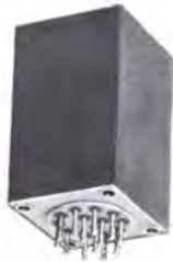
Two self saturating magamps in one case. Output 250 V. into 750 ohms. Power gain 135,000. MIL-T-27C; 2 x 2 x 2½, 12 oz.
