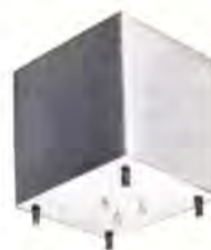
High pass filter, 30 Hz, used to eliminate from the output, 25 Hz sine wave pulses which control automatic programming on audio tracks of music tapes. Flat to 1 db from 50 Hz to 15 kHz, within 3 db to 30 Hz. Attenuation of at least 35 db from 25 Hz to 20 Hz. Source and load 600 ohms. Wt. approx. 6 lbs. MIL-F-18327C.
