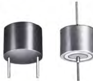
Type FD, 2 microhenry temperature stable miniature inductor. High Q in the 2 MHz to 20 MHz frequency range. Supplied in either epoxy case (23/32 dia x 1/2" high) Grade 5 or metal case (11/16 dia x 9/16" long) Grade 4. MIL-T-27C.
