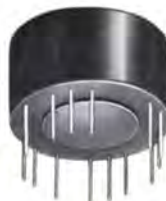
Self-saturating inverter transformer; 100 V DC input. Frequency of oscillation 20 kHz. MIL-T-27C, Class T. Size: 1.25 Dia x .60 H, PC mounting.
