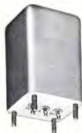
Band reject filters (two shown). The 1050 Hz filter has 50 db attenuation at center frequency and is only 3 db down at 950 and 1150 Hz. The 12.75 kHz filter has more than 100 db attenuation at center frequency and is only 3 db down at 10.8 kHz and 15 kHz. Source and load for each filter 600 ohms, both are MIL-F-18327C. Wt. 0.7 lbs.
