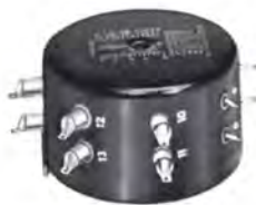
Toroidal Transistor inverter transformer. Input 24 V DC, outputs 4 windings 150 V to 1050 V DC. Hipot 3800 V. Hermetically sealed, MIL-T-27C, 2½ dia. x 1½, 15 oz.
