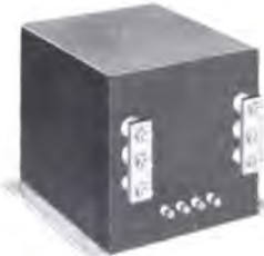
High current filament transformer. Primary 140/156 V., 47/63 Hz to 1.8 V.-1070 A. Current limiting through separate primary reactor, MIL-T-27C; 10 x 10 x 11½", 150 lbs.
