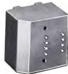
Dual saturable reactor. Input 10 V. - 1 kHz. Output 3.5 V. 2 MA DC control current. 130° C. MIL-T-27C; 1¾ x 1¾ x 1¼, 5 oz.
