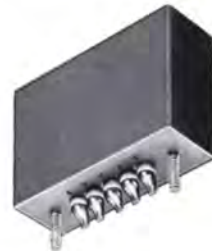
Saturable reactor. Input 50 V.-60 Hz. Output 10 V., 4 MA DC control current. MIL-T-27C; 7/8 x 2½ x 1½, 6 oz.
