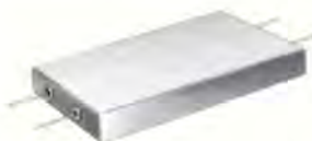
Ultra-miniature low pass filter only 1/4" high. DC to 40 kHz within \pm 0.1 db, within 1 db to 60 kHz, 3 db to 70 kHz. Attenuation of at least 40 db above 81 kHz. Source and load 1K ohms, MIL-F-18327C. Wt. 1.2 ounces.
