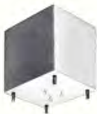
One Hz low pass filter. Flat to 1 db up to 0.75 Hz, within 2 db up to 1 Hz. Attenuation of at least 40 db for frequencies above 2 Hz. Source and load 10K ohms. MIL-F-18327C. Wt. 6 lbs.
