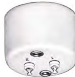
Constant 20 millihenries inductor. Inductance variation less than 2% from 0.1 to 500 V at 100 kHz. Q at 1 volt 100 kHz greater than 100. Case size: 1 1/8 O.D. x 1 3/16" high. MIL-T-27C.
