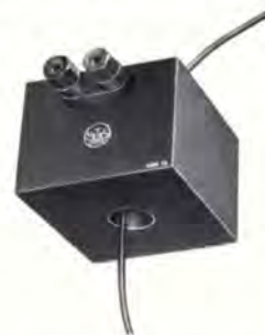
Current Transformer with 1 K load exhibits 1 V/amp/turn sensitivity. From 400 Hz to 30 kHz, \pm 0.1 db. Good linearity with both current, 1 mA-10 A; and turns, 1-5 T.
