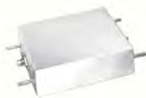
Low pass filter, 6 MHz. DC to 6 MHz within \pm 0.1 db. Attenuation at least 40 db at 8.5 MHz and higher. Source and load 75 ohms. Wt. approx. 8 oz.
