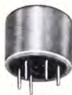
Molded carrier frequency transformer, + 8 dbm level. Within 3 db from 100 Hz to 100 kHz. 4000:4000 ohms. \frac{3}{4} Dia. x \frac{5}{8} inches, \frac{1}{3} oz.
