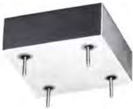
Flat low frequency 50 henries inductor only .400 high. Q of 10 at 100 Hz. DCR 2360 ohms. Grade 4, MIL-T-27C.
