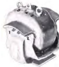
High voltage filament transformer. Primary 115 V., 380/1600 Hz to 5 VCT-10 A., 21 KV hipot. 160° C. MIL-T-27C Grade 5; 2¼ x 2½ x 2¼", 10 ounce.
