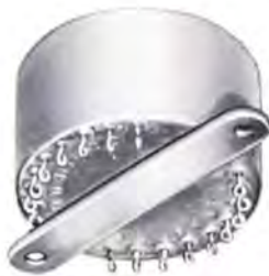
Multi Control Magamp. Power gain 400,000. Control Current .00003A. Output 25 V. DC into 1K. Six power windings, bias, feedback, and two control windings. MIL-T-27C; 2¼ dia. x 1¼ high, 8 oz.
