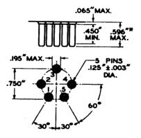
Base-pin positions are held to tolerances such that entire length of pins will enter flat-plate gauge (JETEC No.GA5-1) having thickness of 1/4" and five holes with diameters of 0.1360"  $\pm$  0.0005" so located on a 0.7500"  $\pm$  0.0005" diameter circle that the distance between centers of the four adjacent holes is 0.3750"  $\pm$  0.0005" and the distance between the center of the remaining hole and its adjacent hole centers is 0.5300"  $\pm$  0.0005".
