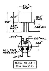
Base-pin positions are held to tolerances such that entire length of pins will enter flat-plate gauge (JETEC No.GA3-1) having thickness of 1/4" and three holes with diameters of 0.1030"- 0.1035" so located on a 0.3440" ± 0.0005" diameter circle that the distance along the chord between
