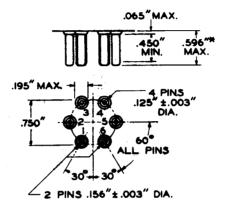
Base-pin positions are held to tolerances such that entire length of pins will enter flat-plate gauge (JETEC No.GA6-I) having thickness of 1/4" and six holes, two adjacent with diameters of 0.1650"  $\pm$  0.0005" and four with diameters of 0.1360"  $\pm$  0.0005" so located on a 0.7500"  $\pm$  0.0005" diameter circle that the distance between any two adjacent hole centers is 0.3750"  $\pm$  0.0005".
