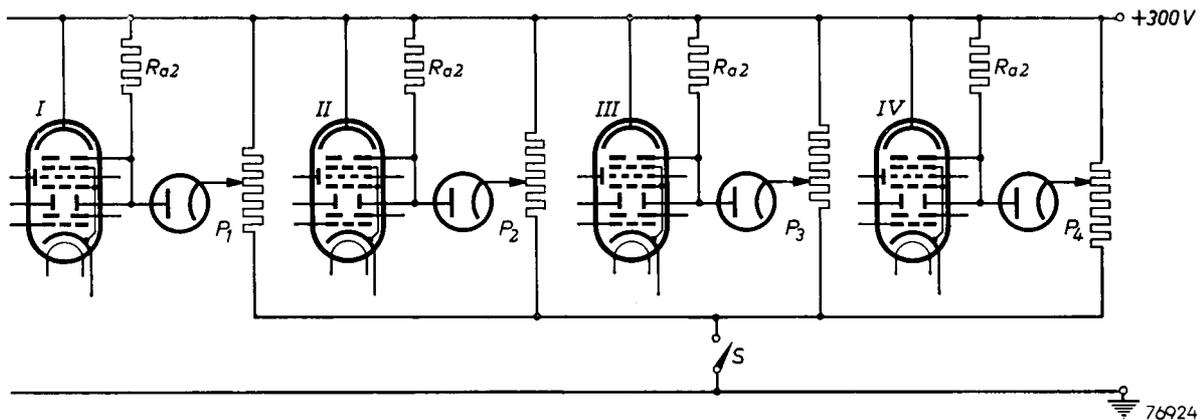
Fig. 22. Basic circuit of a four-decade predetermined counter. In order to obtain a cycle of 7236 counts (i.e. the complementary of  $10\,000 - 7236 = 2764$ ), the potentiometers  $P_1 - P_4$  must be so adjusted that the counter tubes  $I - IV$  are preset to figures 4, 6, 7 and 2 respectively.
