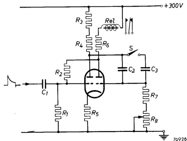
**Fig. 26.** Circuit of an output stage. The time during which the relay *Rel* remains energised when a pulse is fed to the input depends on the values of  $R_8$  and the coupling capacitance between the two triode sections of the E90CC.
