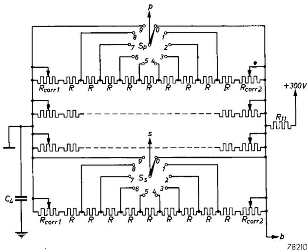
**Fig. 25.** Circuit for replacing the four wire-wound potentiometers  $P_1—P_4$  and the resistors  $R_1—R_{10}$  shown in fig. 6 by fixed resistors  $R$  ( $4.7\text{ k}\Omega \pm 2\%$ ,  $\frac{1}{4}\text{ W}$ ) and four ten-way switches  $S_p—S_s$ . The variable resistors  $R_{corr}$  need be readjusted only when the tubes are replaced. They may be of the carbon type and should have a value of  $10\text{ k}\Omega$ . Only two of the four branches have been completely drawn.
