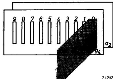
Fig. 3. Diagrammatical representation of a ribbon-shaped beam  $b$  sweeping over a slotted electrode  $g_4$  interposed between the cathode and the anode  $a_2$ .
