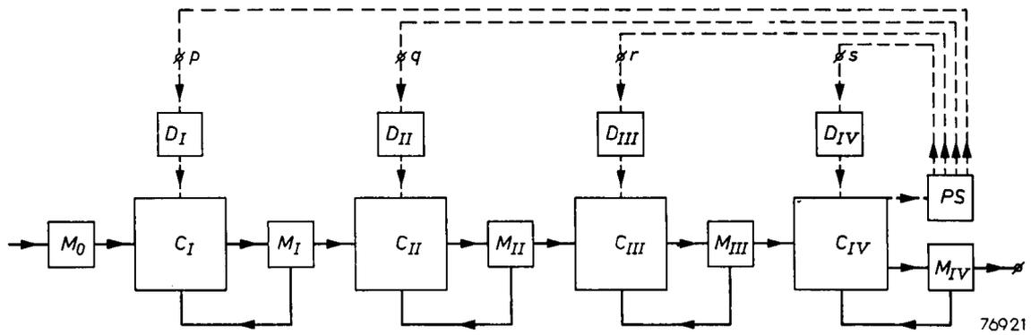
Fig. 19. Block diagram of a four-decade counter.  $C_I$  to  $C_{IV}$  — counter stages,  $M_0$  — input stage,  $M_I$  to  $M_{IV}$  — inter-stage pulse shapers. By adding the presetting stage  $PS$  and the four diodes  $D_I$  to  $D_{IV}$  the circuit can be converted into that of a predetermined counter.
