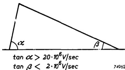
Fig. 7. Required form of the positive pulses to be applied to the left deflection electrode. The slope of the leading edge should be at least  $20 \times 10^6$  V/sec, that of the trailing edge should not exceed  $2 \times 10^6$  V/sec. The average amplitude of the pulse should be 13.6 V.
