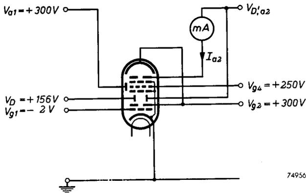
Fig. 2. Circuit for measuring the  $I_{a2} = f(V_{D',a2})$  characteristic.
