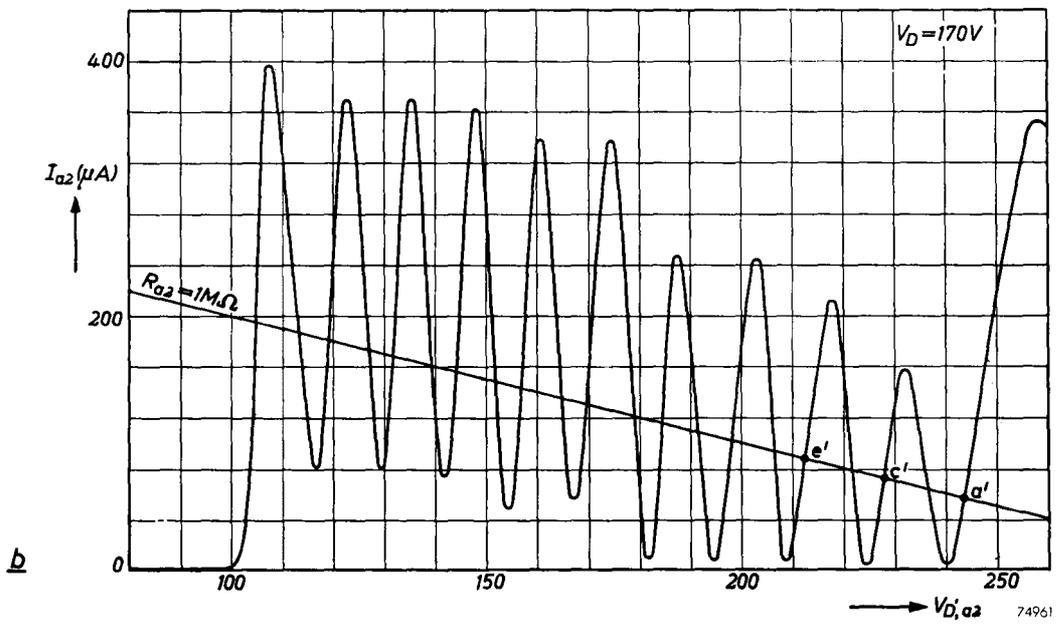
Fig. 6.  $I_{a2} = f(V_{D, a2})$  characteristic for a left deflection electrode voltage  $V_D = 156\text{ V}$  (a) and for  $V_D = 170\text{ V}$  (b).
