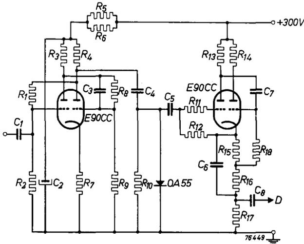
Fig. 12. Input pulse shaper with auxiliary pulse shaper.
