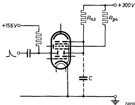
Fig. 5. Circuit for explaining the operation of the EIT counter tube, positive voltage pulses being applied to the left deflection electrode. *C* represents the sum of the capacitance of the anode and of the right deflection electrode with respect to all other electrodes and the wiring and stray capacitances.
