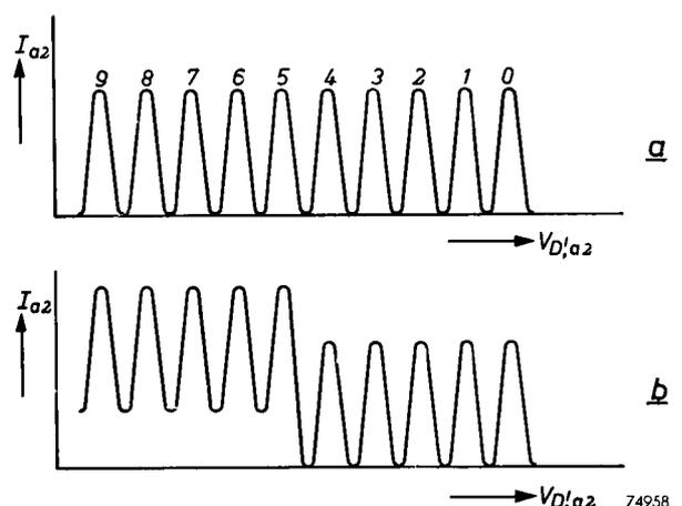
Fig. 4. (a) Hypothetical  $I_{a2} = f(V_{D',a2})$  characteristic of a tube provided with a slotted electrode  $g_4$  with identical, equidistant slots according to fig. 3. (b) As fig. 4a, but taking into account the presence of a horizontal slot at the bottom left.
