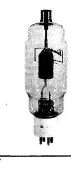
Heat Dissipating Connector or equivalent is required on the plate terminal.
