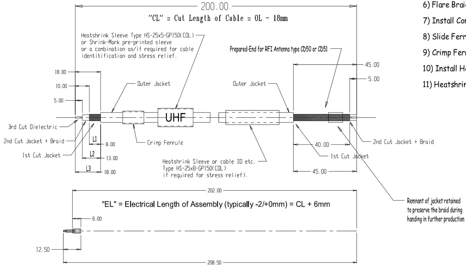
$$\text{"EL"} = \text{Electrical Length of Assembly (typically } -2/+0\text{mm)} = \text{CL} + 6\text{mm}$$
