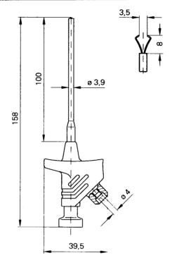
Clamp-type test prod with rotating gripper and flexible shaft. The gripper has been specially shaped so that pins and wires up to a maximum diameter of 4 mm can be connected without slipping off. Connectors and wires measuring up to 4 mm in diameter can be connected with the aid of the 4 mm dia. socket connection with lateral screw. Socket made of brass, gripper additionally nickelplated.
