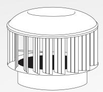
An area of low pressure is created on the leeward side of the vent and the air drawn out between the vanes on the head of the ventilator feeds this low pressure zone. This process allows for a continuous air flow through the vent.
