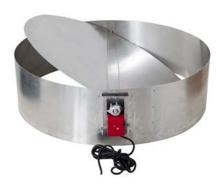
This Damper System can be used with the Roofquip straight Vane Ventilators where the ventilation performance may need to be reduced at certain times. The system offers the ability to stop at any position whilst opening or closing. There is a gap of approx 12mm around the circumference of the damper blade to allow some air flow through the ventilator at all times.
