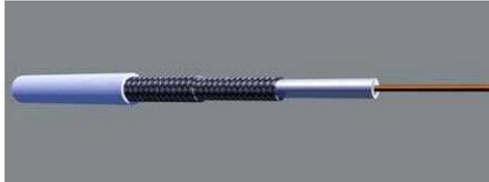
The cable consists of a plain annealed copper inner conductor coated with a solid polyethylene dielectric Type 03 to BS6234, surrounded by two layers of braided copper wires and sheathed with polyvinyl chloride, Type TM1 to BS7655. Low Smoke Zero Halogen sheath option is also available.
