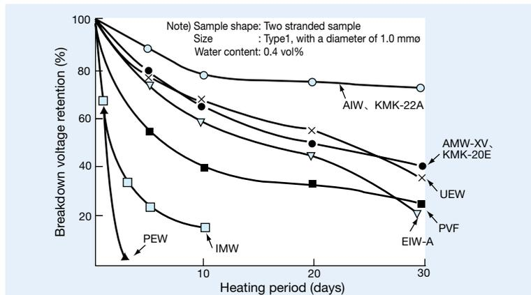
● Table 4: Example of charge water resistance (Type1, with a diameter of 1.0 mm)
