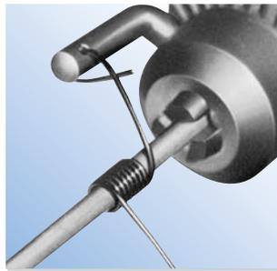
● Figure 2: Winding Test
