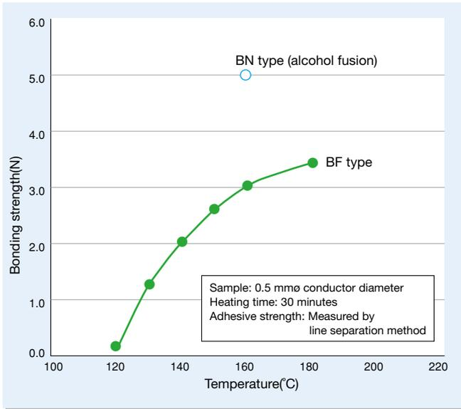
● Figure 11: Bonding characteristics of self-bonding wire in high temperatures
