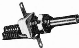
Type C.1604. Miniature Trimmer. Same construction as the Type C.16 but provided with \frac{1}{4} " x 40TPI Bush and Lock Nut for single hole mounting. Shaft diameter \frac{5}{32} ". Page 51
