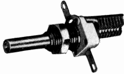
Page 51 Type C1604. Miniature Trimmer. Same construction as the Type C16 but provided with \frac{1}{4} " x 40TPI Bush and Lock Nut for single hole mounting. Shaft diameter \frac{3}{32} ".
