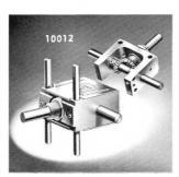
worm DRIVE UNIT — Cast aluminum frame may be panel or base mounted. Spring loaded split gears to minimize back lash. Standard ratio 16/1. Also in 48/1, 36/1, 12/1. No. 10000 — (state ratio)
