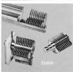
12000 SERIES TRANSMITTING CAPACITORS — Rigid heavy channeled aluminum end plates. Ceramic insulation, polished or plain edges. One piece rotor contact spring and connection lug. Compact, easy to mount with connector lugs in convenient locations.
