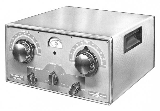
The **No. 92200 Transmatch** is a 2 KW band-switching, adjustable r.f. transformer with a reflectometer as the indicator. The **Transmatch**, inserted between a transmitter and a transmission line, will convert the impedance of any 15 to 500 ohm coaxial fed antenna system to 50 ohms so that the transmitter may, at all frequencies, work into the impedance for which it was designed.
