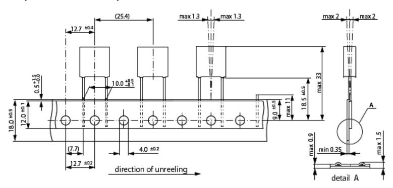
The original lead spacing of 15.0 mm (suffix code — T2) (the pitch of holes on carrier tape = 12.7 mm) (All dimensions in mm)
