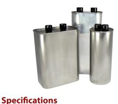
Type HV capacitors are constructed with low loss self healing metallized polypropylene film. Packaged in a cylindrical, oval and rectangular metal cases. Type HV capacitors are ideal for AC filtering, CVT filtering/snubbering, line current reduction and voltage regulation in power supply applications.
