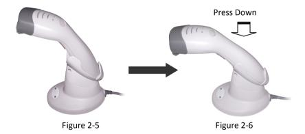
Once the scanner is well situated in the cradle, press down any one of the small buttons at the side of cradle LED lamp to start charging (Shown as Figure).
