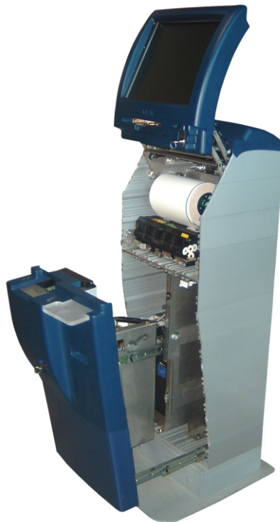
Full access to all internal components for quick, cost-effective service
