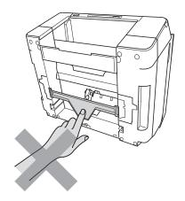
DO NOT carry the machine by holding the scanner cover or the Jam Clear Cover. Doing this may cause the machine to slip out of your hands. Only carry the machine by placing your hands under the entire machine.
