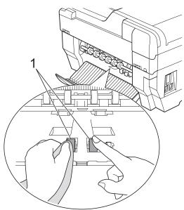
5 Clean the Back Paper Feed Rollers (1) with a soft lint-free cloth moistened with water.
