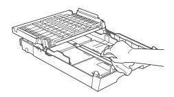
5 Close the output paper tray cover and put the output paper tray firmly back in the machine.
