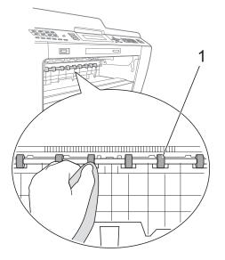
3 Lift the Jam Clear flap (2), and then clean the back side of the Paper Feed Rollers (1) with a soft lint-free cloth moistened with water.
