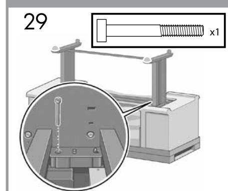
**EN** Use one screw to attach the right side of the stand to the printer engine. Make sure that the screw is fully tightened.
