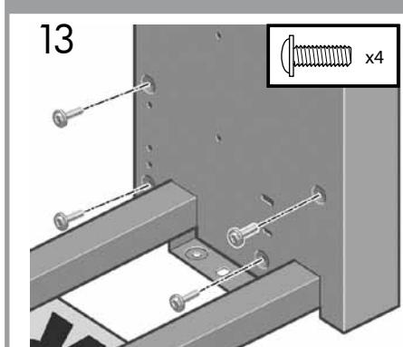
**EN** Use four screws on the inside of the right leg to attach the right leg to the cross-brace.
