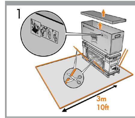
**EN** Cut the straps, open the box and remove the top cover and the box from the printer.
