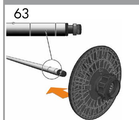
**EN** Slide the black hub onto the spindle up to one of the two marks.
