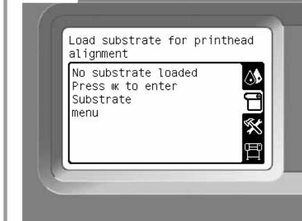
From the front panel, select the substrate icon and then press the OK button.
