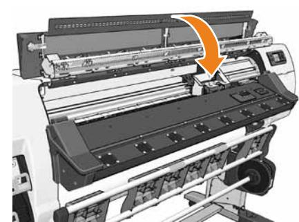
Close the printer window and secure the latches.
