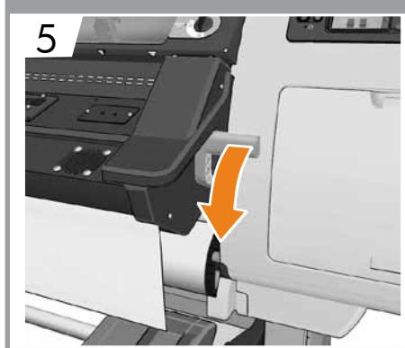
**EN** Lower the substrate-adjustment lever.
