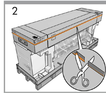
Carefully cut the straps around the boxes. Make sure that the boxes don't fall when the straps are cut.
