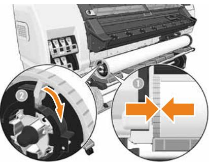
**EN** Slide the blue hub onto the spindle. Make sure that the blue hub is fully inserted into the roll of substrate (no gap should exist between the hub and the roll), and then lock the hub.
