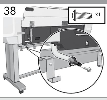
**EN** Screw the printer tube to the stand.
