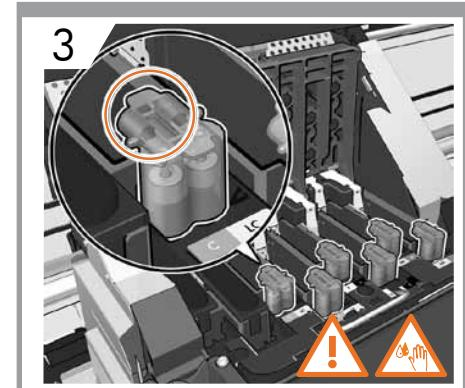
Check that all setup printheads have ink, if not then repeat step 1. If a system error appears, contact support.
