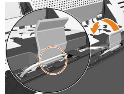
Lower and lock the blue latch. Make sure that the blue latch is correctly engaged, and then lower the latch.
