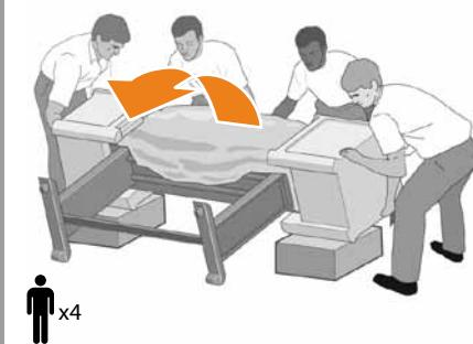
**EN** Use the hand holds at the rear of the printer engine to carefully lift the printer to its upright position. HP recommends four people to complete this task.
