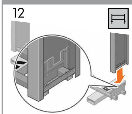
**EN** Lower the right leg onto the right side of the cross-brace. The right leg will fit only on the right side of the cross-brace.
