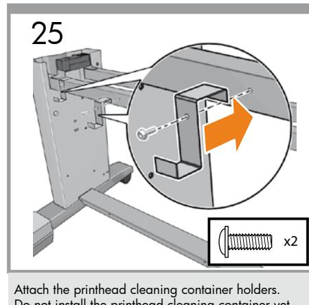
**EN** Attach the printhead cleaning container holders. Do not install the printhead cleaning container yet.
