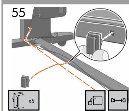
**EN** Use the clips provided to attach the sensor cable to the lower cross-brace.
