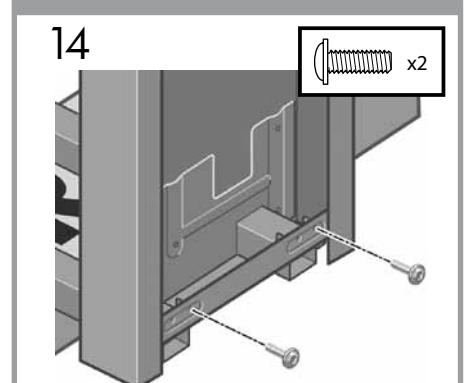
**EN** Use two screws on the outside of the right leg to attach the left leg to the cross-brace.
