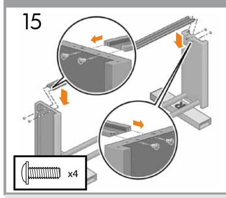
**EN** Use four screws to attach the cross-bar to the legs.
