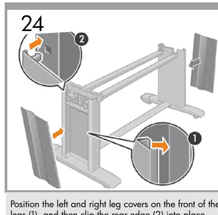
**EN** Position the left and right leg covers on the front of the legs (1), and then clip the rear edge (2) into place.
