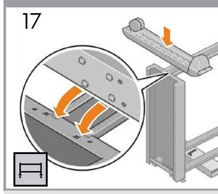
**EN** Place a foot on the left leg. There are pins to help you correctly position the foot. Do not remove the anti-slip material from the wheel.
