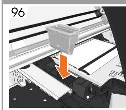
**EN** Insert the ink funnel (located inside the maintenance cartridge box ) into position.
