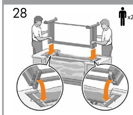
**EN** Lift the stand assembly onto the printer engine. The anti-slip material should face the rear of the printer. Check that the tube from container does not interfere with the stand and printer.
