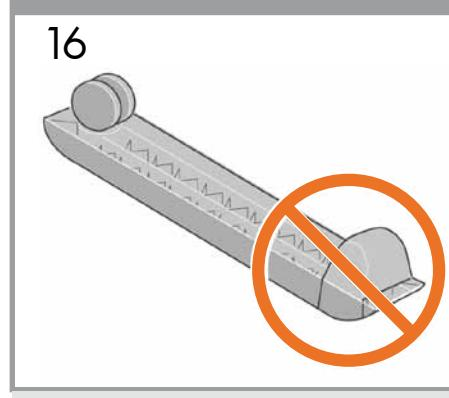
**EN** Notice that there is anti-slip material around two of the wheels on the feet. DO NOT REMOVE this material yet.
