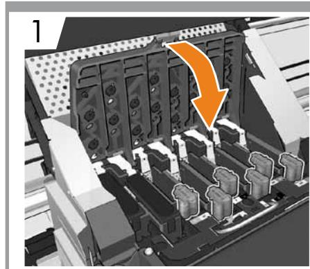
**EN** Do not remove the setup printheads, close the carriage cover and the printer window.
