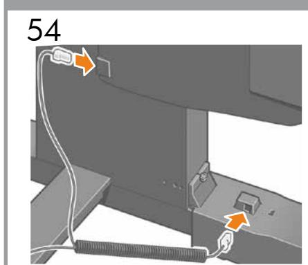
**EN** Connect the sensor cable to the rear of the take-up reel motor. Connect the sensor cable to the sensor unit located on the right foot.
