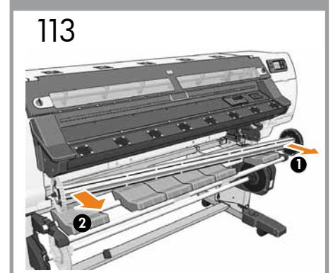
Remove the spindle from the printer.
