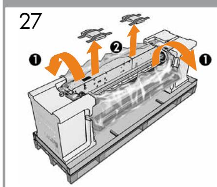
**EN** Pull open the protective plastic from the base of the printer (1), and then remove the two desiccant bags (2).
