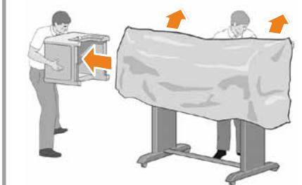
**EN** Remove the two foam end-packs, and then remove the plastic covering from the printer engine.
