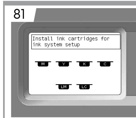
**Wait until this message appears. The front panel guides you through the procedures for inserting the ink supplies. Note: Ink supplies are not provided with the printer.**
