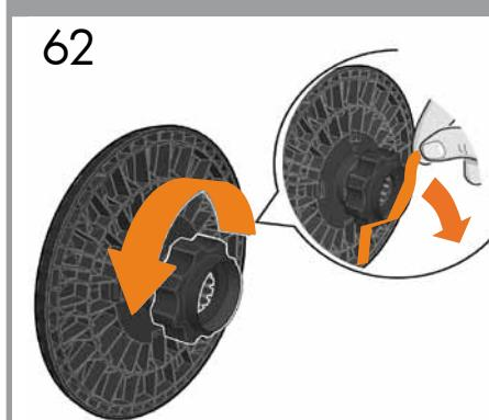
**EN** Remove the adhesive tape, and then loosen the plastic nut on the black hub.
