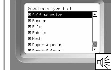
On the front panel, select the family of the substrate roll you loaded into the printer, and then press the OK button.
