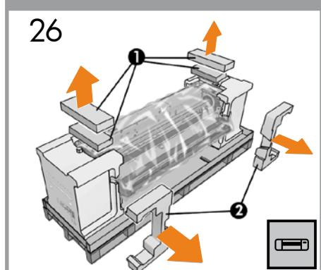
**EN** Remove the four packing pieces from the top (60-inch printer only) and two pieces from the side as shown.
