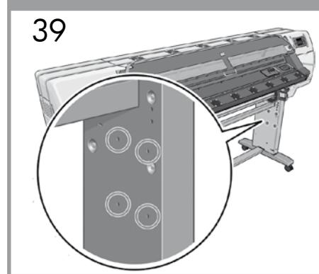
Identify the four holes on the inside of the right leg. The holes are used to attach the take-up reel motor.
