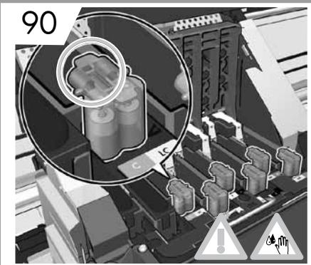
Before removing the setup printheads, look at each printhead and verify that each printhead contains ink.
