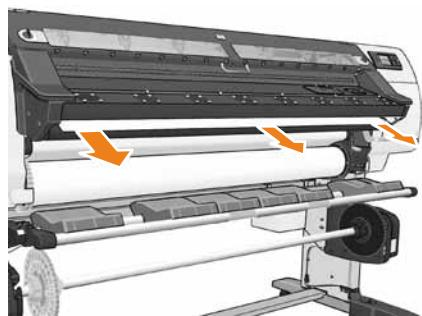
Wait until the substrate emerges from the printer as shown.
