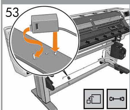
**EN** Attach the sensor unit onto the left side of the lower cross-brace.
