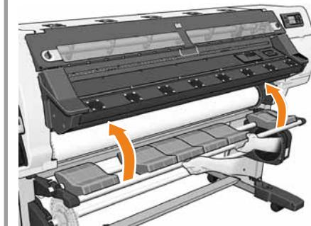
With the blue hub on the left, lift the loading table to ease the spindle into the printer.
