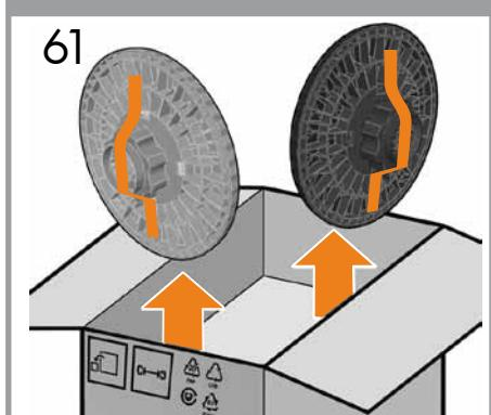
**EN** Remove the two take-up reel hubs.
