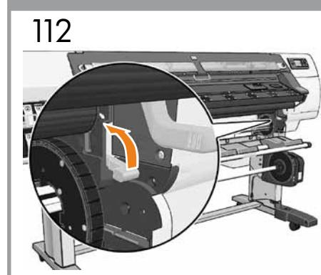
Remove the adhesive tape, and lift the spindle lock lever to disengage the spindle.
