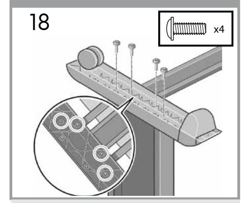
**EN** Use four screws to attach the foot to the left leg. Tighten each screw half-way, and then gradually tighten each screw completely.
