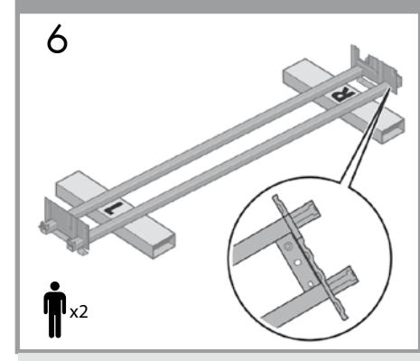
**EN** Lower the left side of the cross-brace onto the box marked L and the right side of the cross-brace onto the box marked R.
