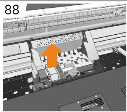
Remove the packing foam from the top of the printhead carriage.
