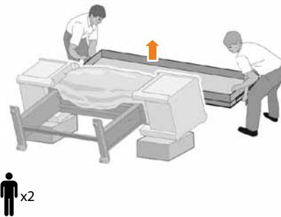
**EN** Remove the pallet before lifting the printer to its upright position.
