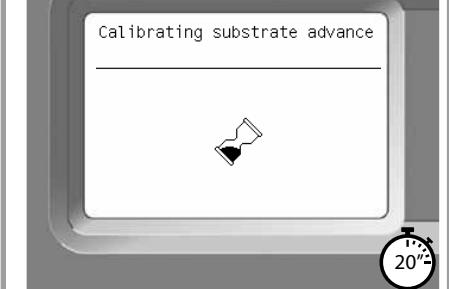
The printer automatically performs substrate advance calibration and printhead alignment. Please do not stop those processes to ensure successful PH alignment.
