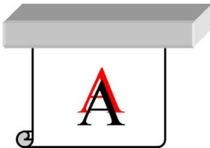
If the colors are misaligned in any direction, the printheads may be misaligned. This is likely if you have not aligned the printheads for a long time, or if there has been a substrate jam. Align the printheads if necessary (see [Align the printheads on page 11](#)). You can check whether it is necessary by using the printhead status plot (see [Use the printhead status plot on page 22](#)).
