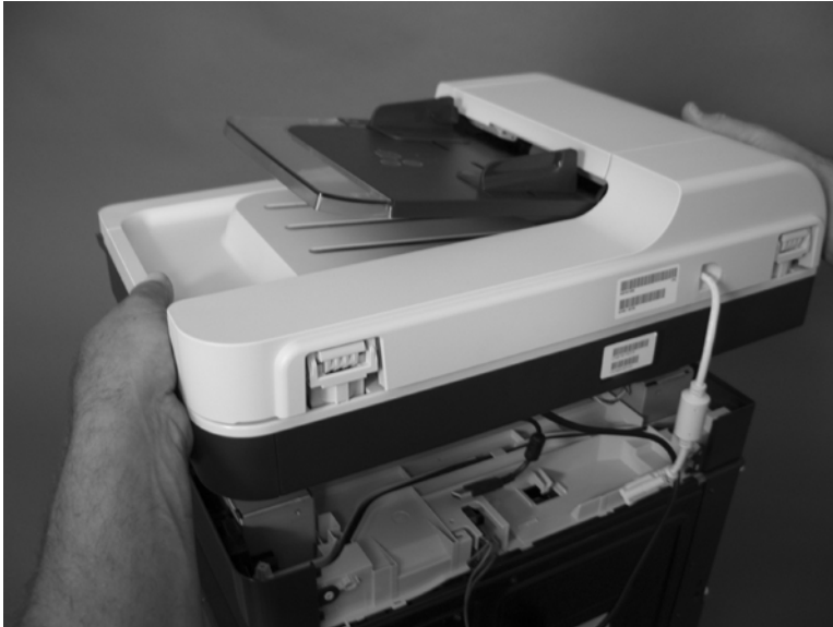
Figure 6-102 Remove the scanner assembly (6 of 6)
