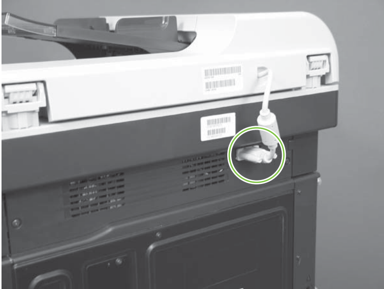
Figure 6-46 Remove the ADF assembly (1 of 4)
