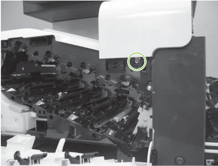
Figure 6-67 Remove the front-upper cover (3 of 4)
