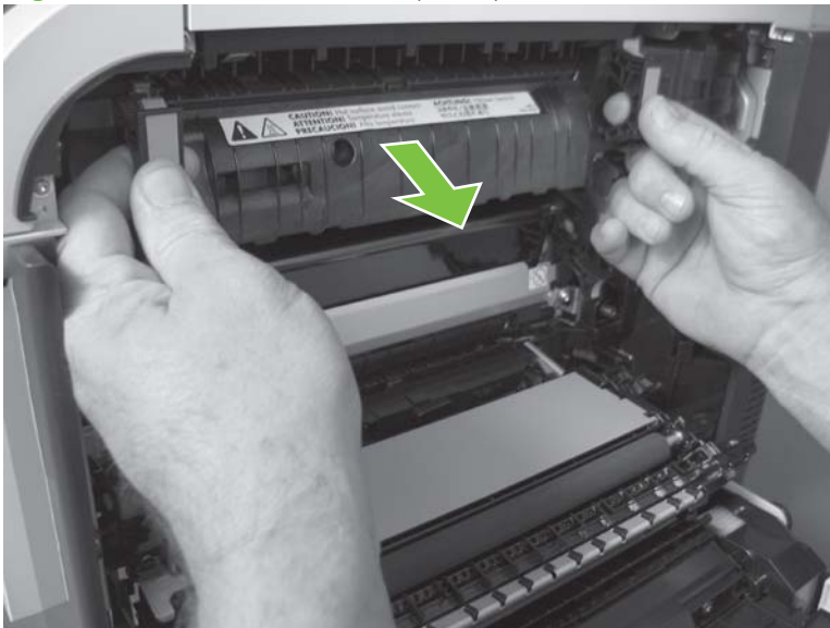
Figure 6-25 Remove the fuser (2 of 2)
