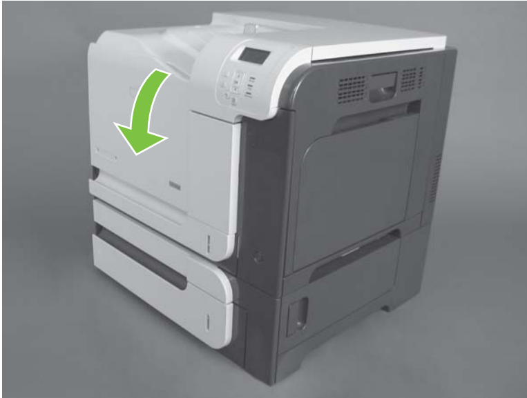
Figure 6-10 Remove the toner-collection unit (1 of 4)
