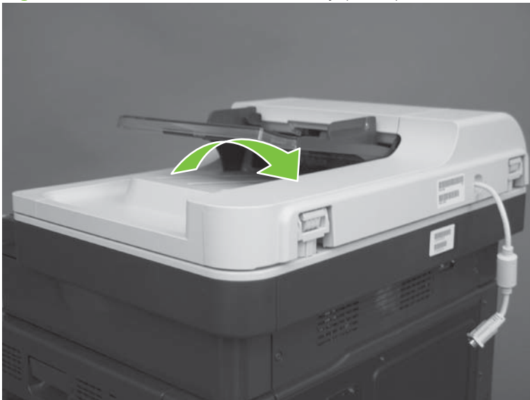
Figure 6-47 Remove the ADF assembly (2 of 4)
