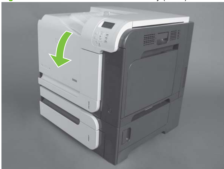
Figure 6-44 Remove the front-door assembly (1 of 2)
