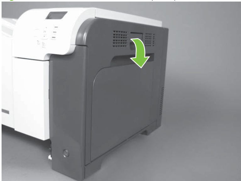
Figure 6-33 Remove the transfer roller (1 of 3)
