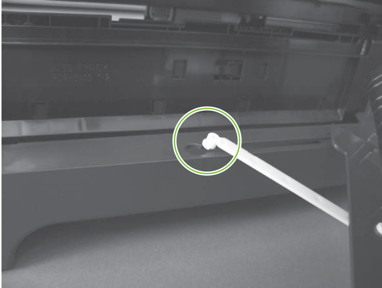
Figure 6-63 Remove the right door; optional paper feeder (3 of 3)
