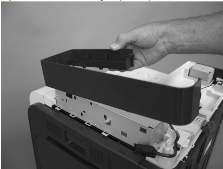
Figure 6-128 Remove the right-top cover (5 of 5)
