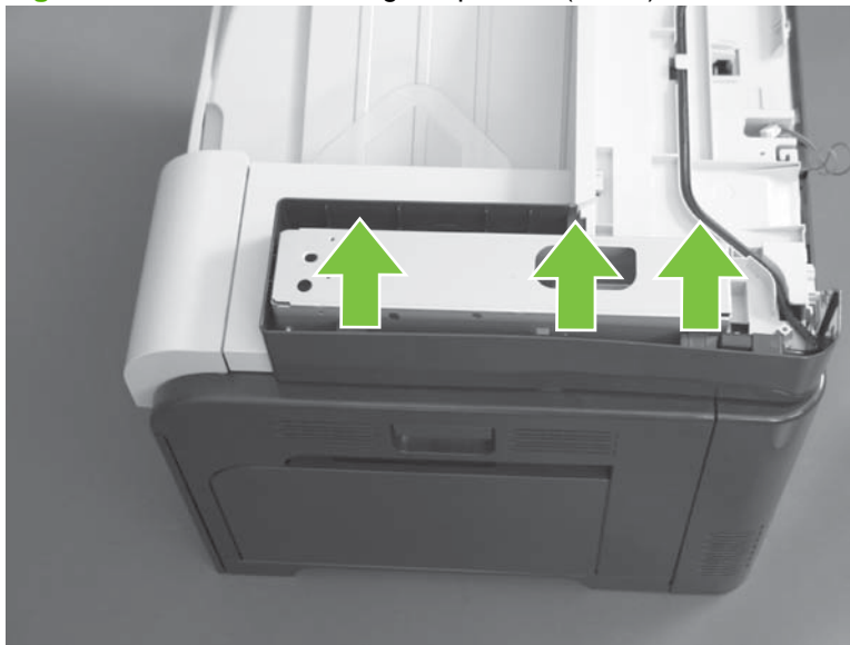
Figure 6-126 Remove the right-top cover (3 of 5)
