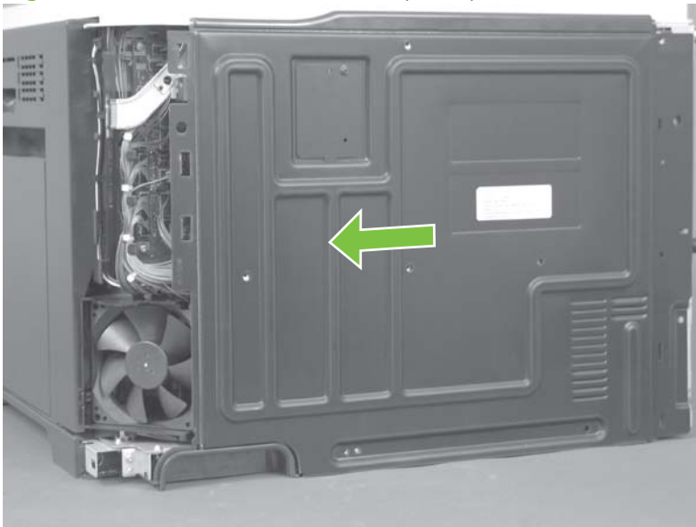
Figure 6-90 Remove the rear cover (2 of 2)
