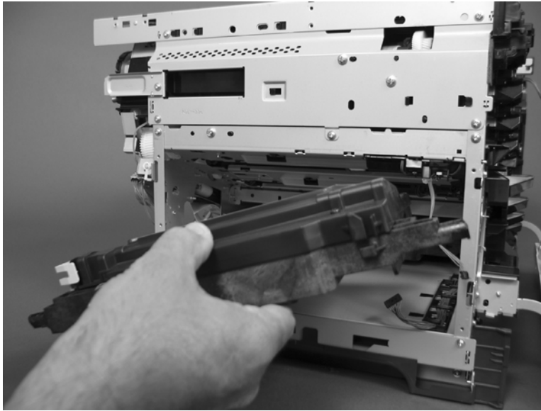
Figure 6-242 Remove the laser/scanner assembly (Y/M) (12 of 12)
