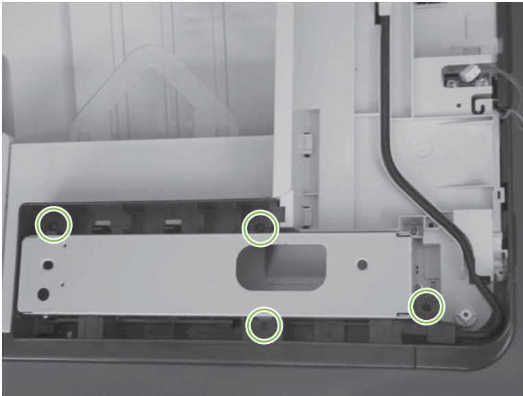
Figure 6-124 Remove the right-top cover (1 of 5)
