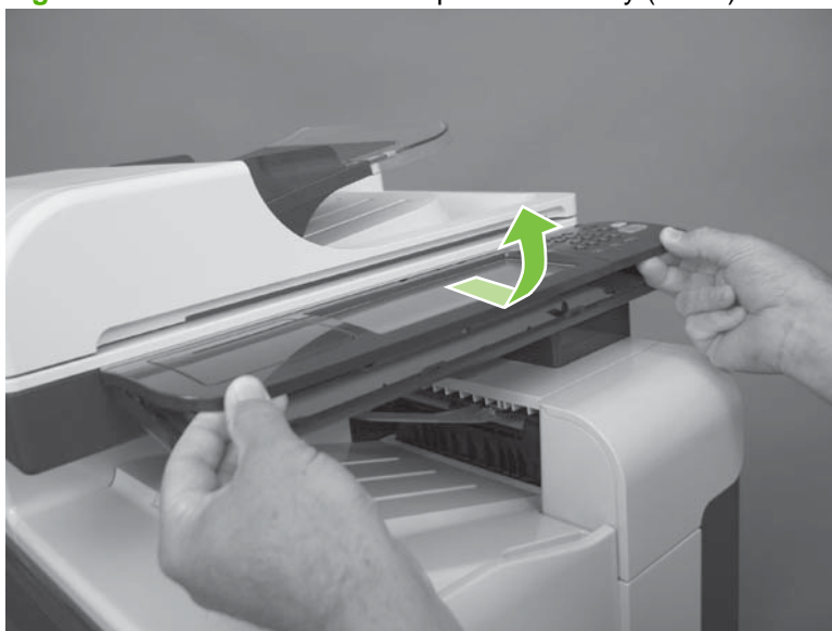
Figure 6-59 Remove the control-panel assembly (2 of 3)
