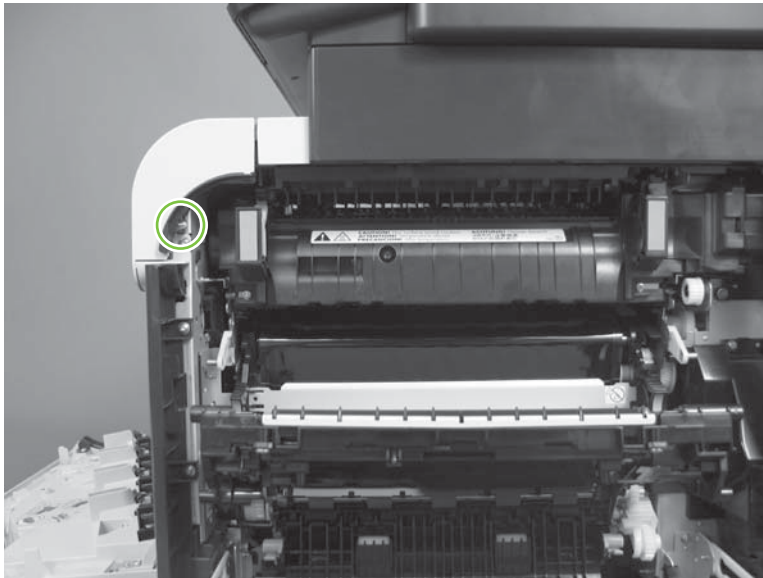
Figure 6-66 Remove the front-upper cover (2 of 4)
