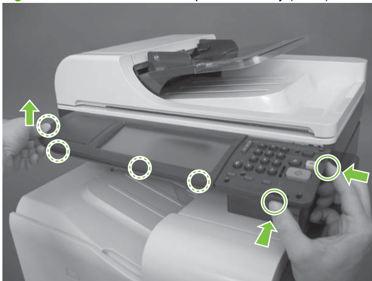
Figure 6-58 Remove the control-panel assembly (1 of 3)
