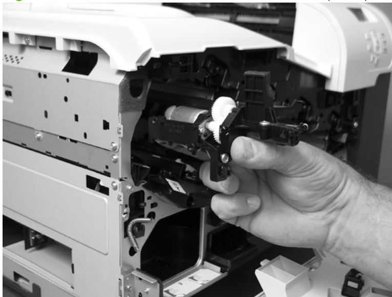
Figure 6-185 Remove the residual-toner-feed motor (7 of 7)
