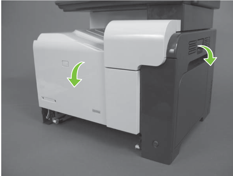
Figure 6-65 Remove the front-upper cover (1 of 4)
