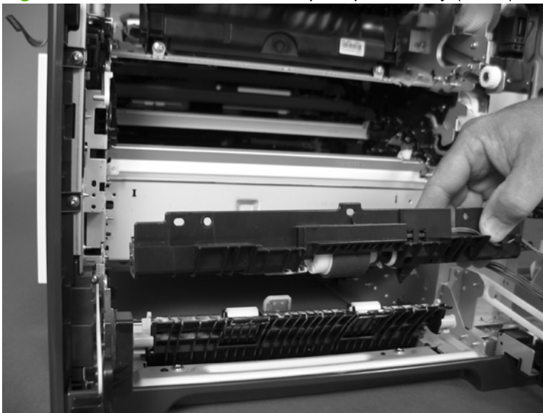
Figure 6-230 Remove the cassette-pickup assembly (3 of 3)
