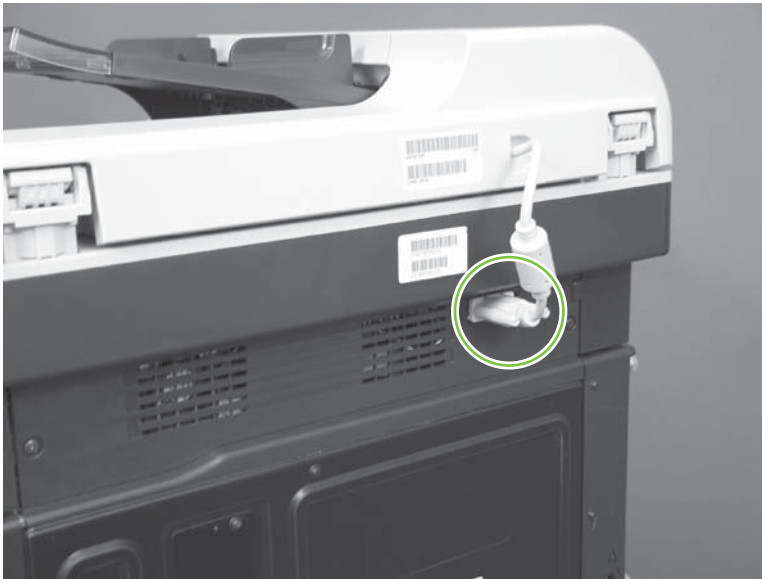
Figure 6-85 Remove the rear-upper cover (1 of 4)
