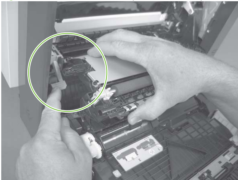
Figure 6-40 Reinstall the secondary transfer assembly
