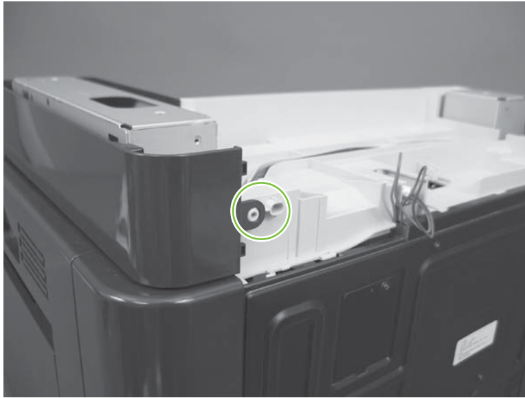
Figure 6-125 Remove the right-top cover (2 of 5)
