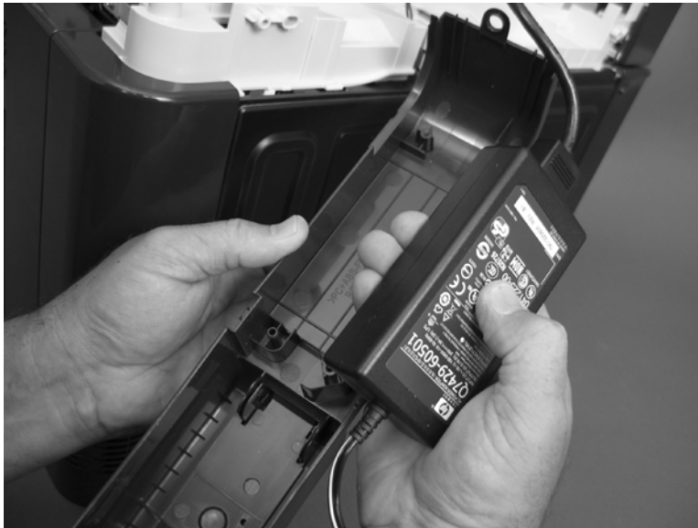
Figure 6-120 Remove the front stapler cover and right-side stapler cover (13 of 13)
