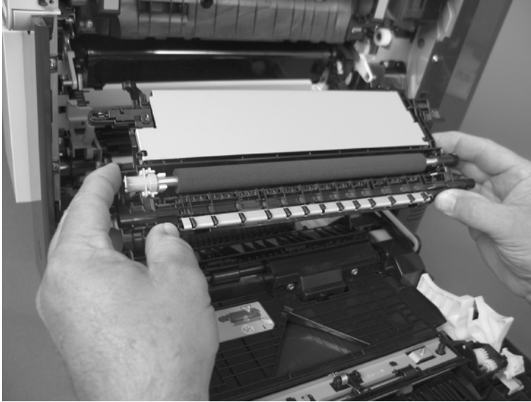
Figure 6-39 Remove the secondary transfer assembly (2 of 2)
