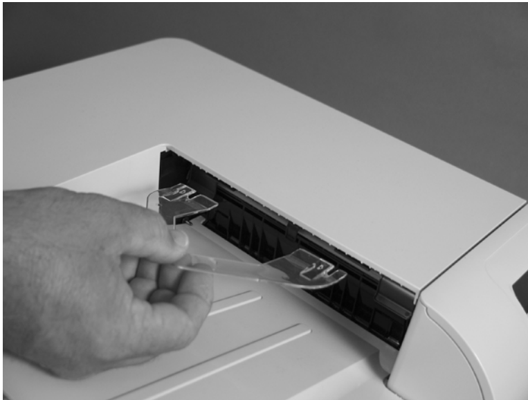
Figure 6-9 Remove the duplex-reverse guide (2 of 2)
