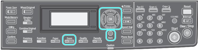
To change a setting, press the [◀], [▶], [▲] or [▼] key in
